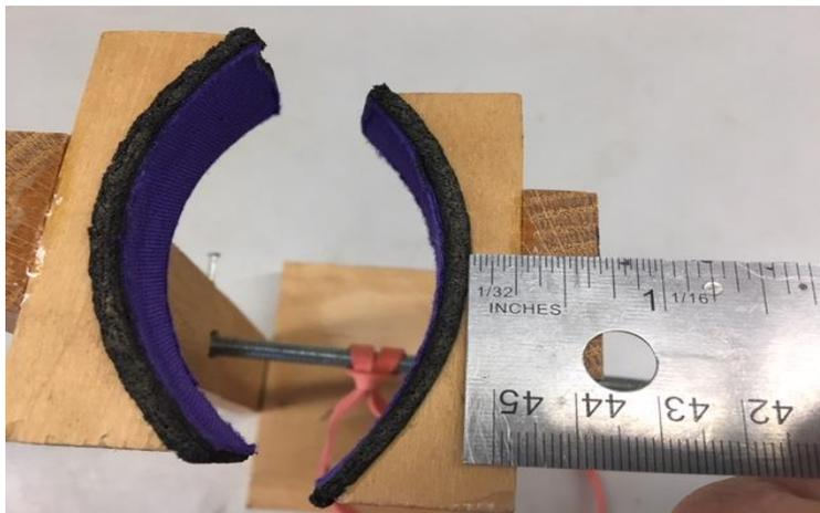
Cut a radius of  $3\frac{1}{2}$  inches into the cup blanks leaving  $\frac{1}{4}$  inch in the middle of the radius and 1 inch at each end as pictured above.
